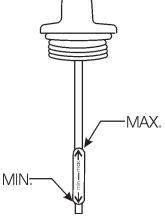
Figure 6. Engine Oil Dipstick (Oil Level)
